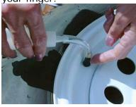
7) Install the filtered valve cores.
